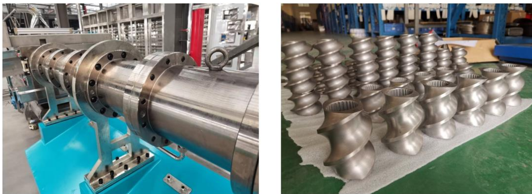
Figure 1: Partial view of the extrusion system and elements of a twin-screw extruder. Source: https://www.indiamart.com/proddetail/extruder-screw-manufacturers-with-profile-ground-23177313048.html .
