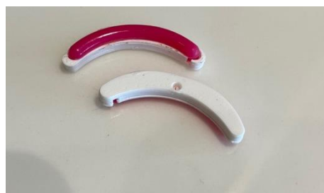
Fig 10: The 3D printed CAM model illustrating the eyelid fasteners (white color) of the proposed tool including the rubber padding (pink color).
