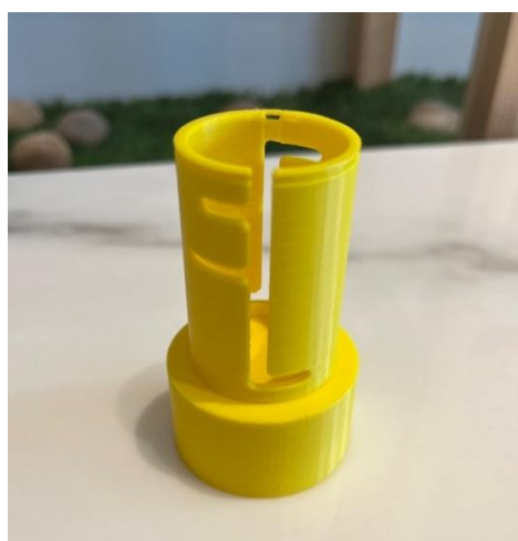
Fig 6: The 3D printed CAM model illustrating the housing of the proposed tool.
