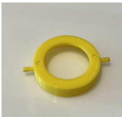
Fig 9: The 3D printed CAM model illustrating the eyelid bracket of the proposed tool.
