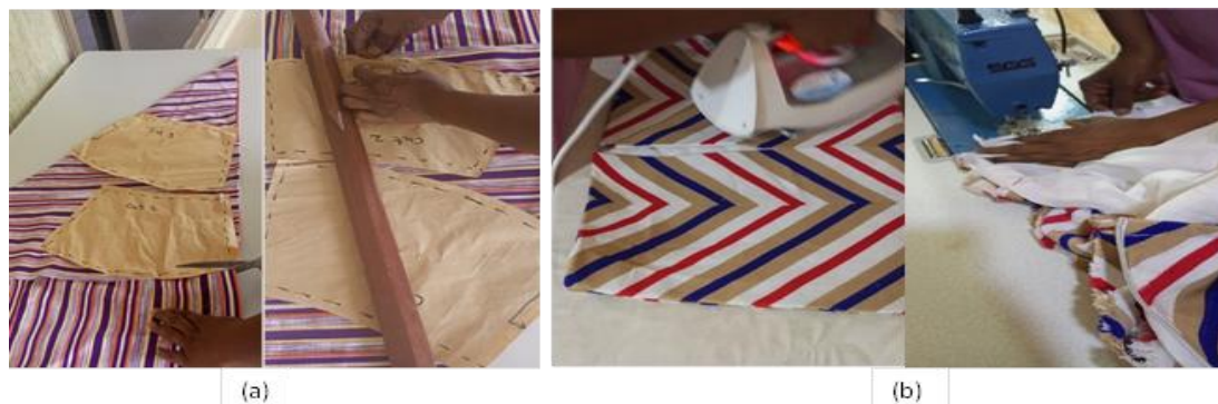
Figure 7 'a': Laying and Cutting of Parts of Garments and 'b' Sewing and Pressing
