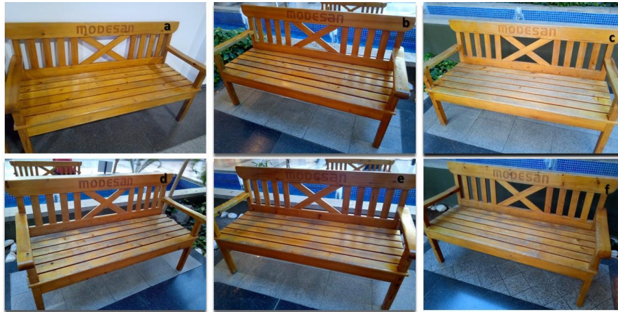
Figure 2: Outdoor exposed some clear coated wooden sitting elements (a, b and c: well protected sitting elements, d, e and f: peeled off transparent sitting units)
