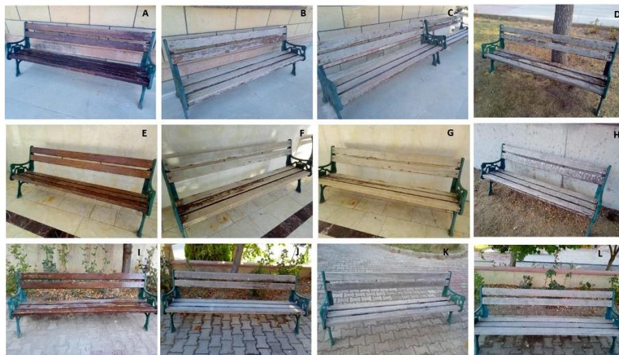
Figure 2: Three sitting units are prepared from the same wooden material and established at the same time in a park. (A, E and I: Painted and aged moderately, B, C, D, E, F, G, H, J, K and L: Painted and aged severely).
