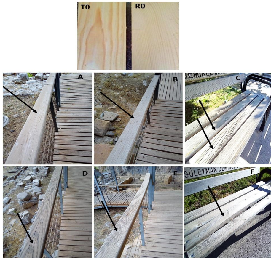
Figure 1: Outdoor exposed surfaces of pine wood samples.
